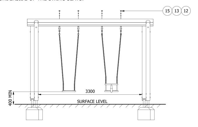
4. FINALLY, ENSURE UNIT IS LEVEL AND PLUMB, ALL FIXINGS HAVE BEEN TIGHTENED AND PROTECTIVE CAPS IN PLACE. ADD CONCRETE TO EACH FOUNDATION HOLE AND
