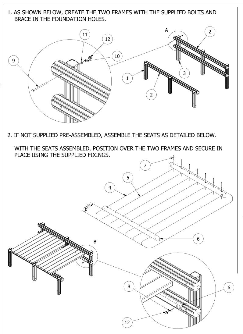
3. FINALLY, ENSURE THE UNIT IS LEVEL AND PLUMB. ALL FIXINGS HAVE BEEN TIGHTENED AND PROTECTIVE CAPS IN PLACE. ADD CONCRETE TO EACH FOUNDATION HOLE AND LEAVE FOR 48 HOURS
