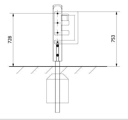
3. FINALLY, ENSURE THE UNIT IS LEVEL AND PLUMB. ALL FIXINGS HAVE BEEN TIGHTENED AND PROTECTIVE CAPS IN PLACE. ADD CONCRETE TO EACH FOUNDATION HOLE AND LEAVE FOR 48 HOURS
