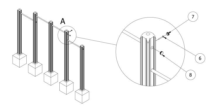
3. FINALLY, ENSURE THE UNIT IS LEVEL AND PLUMB. ALL FIXINGS HAVE BEEN TIGHTENED AND PROTECTIVE CAPS IN PLACE. ADD CONCRETE TO EACH FOUNDATION HOLE AND LEAVE FOR 48 HOURS
