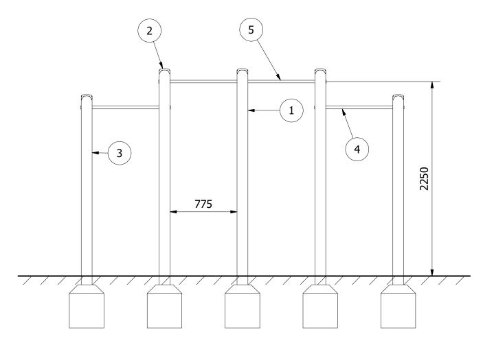
2. FOLLOW THE SAME STEP AS ABOVE, USING PULL UP BAR (ITEM 4) TO CONNECT THE OUTER TIMBERS TO THE CENTRE TIMBERS.BRACE AND SECURE IN PLACE USING THE SUPPLIED FIXINGS AS ILLUSTRATED BELOW.
