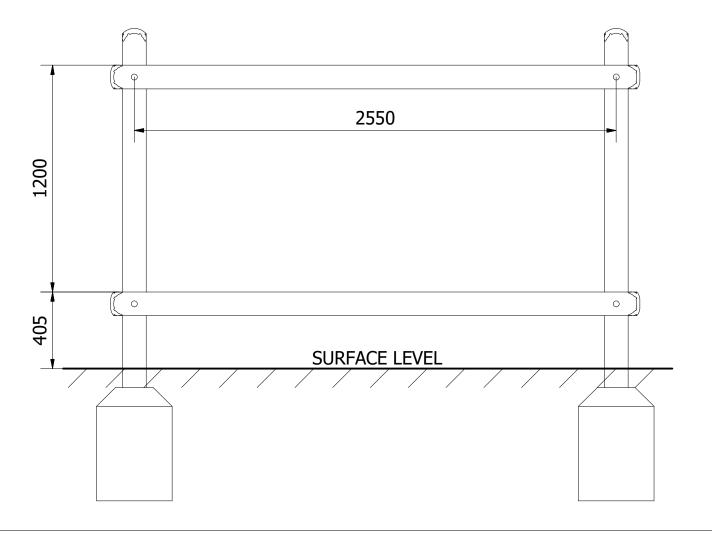
3. FINALLY, ENSURE THE UNIT IS LEVEL & PLUMB, ALL FIXINGS HAVE BEEN TIGHTENED AND PROTECTIVE CAPS IN PLACE. ADD CONCRETE TO THE REMAINING FOUNDATION HOLE AND LEAVE FOR 48 HOURS
