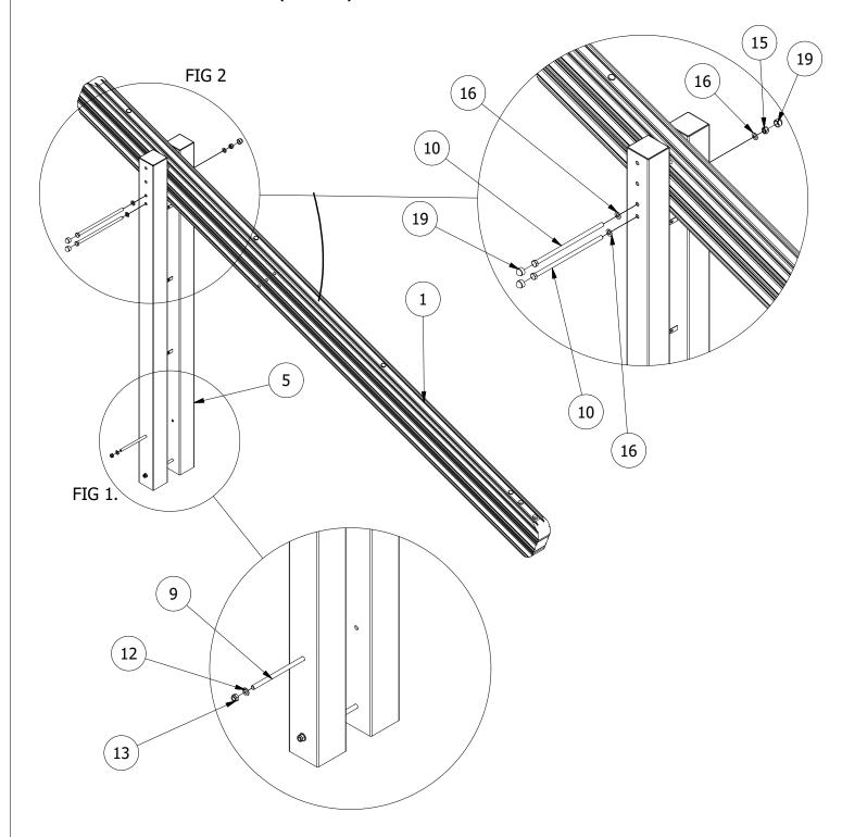
3. POSITION THE TIMBER CROSS BEAM (ITEM 1) RESTING ONTO THE BOLT FROM THE PREVIOUS STEP. SECURE THE NEXT BOLT THROUGH THE STEEL UPRIGHTS AND THROUGH THE TIMBER CROSS BEAM.
