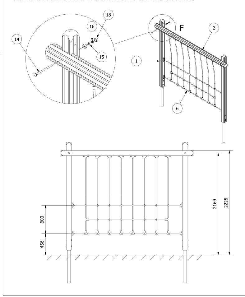
9. FINALLY, ENSURE ALL FIXINGS HAVE BEEN TIGHTENED AND PROTECTIVE CAPS IN PLACE. ADD CONCRETE TO EACH FOUNDATION HOLE AND LEAVE FOR 48 HOURS
