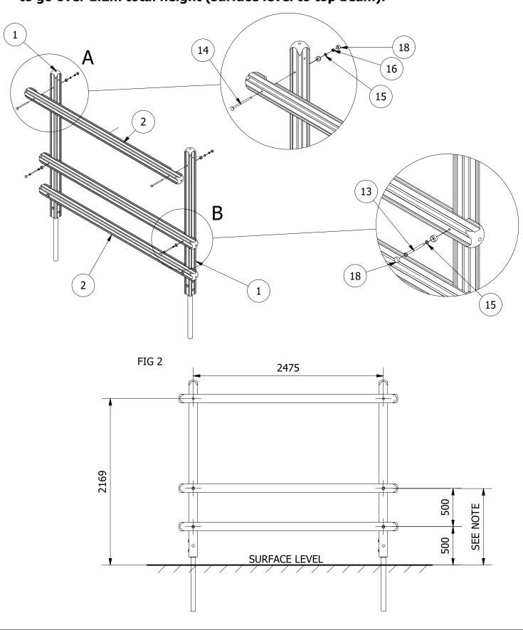
3. POSITION THE PREVIOUSLY BUILT FRAME IN THE FOUNDATION HOLE AND BRACE. ENSURE THE UNIT IS LEVEL AND PLUMB AND ADD RAPID SET CONCRETE TO SECURE.
