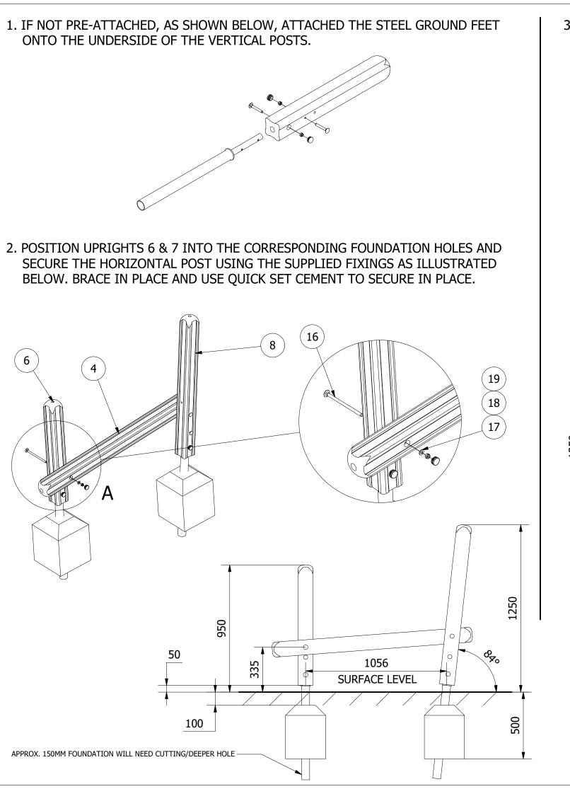
3. WITH PART OF THE UNIT SET IN PLACE, THE REMAINING ITEMS CAN BE POSITIONED INTO THEIR CORRESPONDING FOUNDATION HOLES. USE THE SAME FIXINGS AS THE PREVIOUS STEP - EXCLUSIVE OF THE BELOW TIMBER ITEM 3.
