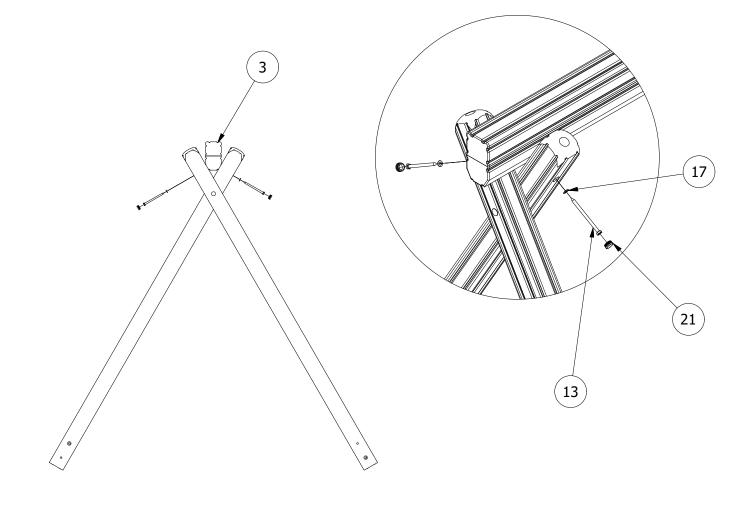
3. AS ILLUSTRATED BELOW, THE TOP CROSSBAR IS SUPPLIED IN TWO PARTS. SECURE THE TWO PARTS TOGETHER AND ATTACH BOTH END A-FRAMES.
