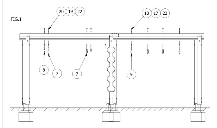
5. HANG THE BIRDS NEST SWING ATTACHING THE SWING CHAIN TO THE SWING HANGERS AND THE SECURITY CHAIN TO THE SWING CHAIN. ENSURE THE SEAT SITS A MINIMUM OF 400MM FROM FINISHED SURFACE LEVEL TO UNDERSIDE OF THE BASKET SEAT/SWING SEATS.
