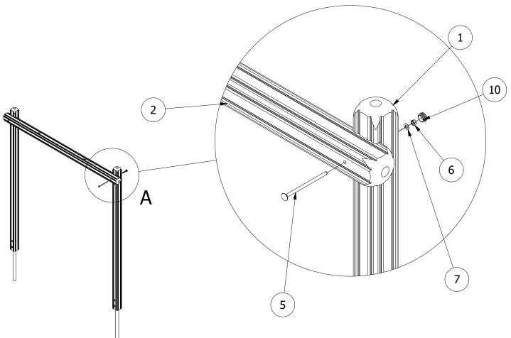
Note: Take extreme care with stainless steel fixings: Use a lubricant/low torque settings before securing with a nyloc nut.
