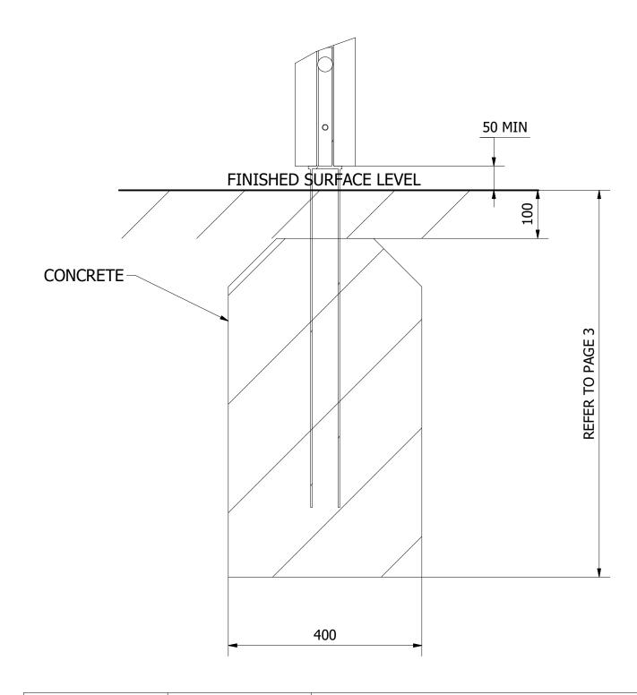
UNLESS OTHERWISE SPECIFIED: DIMENSIONS ARE IN MILLIMETERS PRO-500-130 ROPE CLIMB (FC3) THE INFORMATION CONTAINED IN THIS TOLERANCES: DRAWING IS THE SOLE PROPERTY OF Product Range: FENLAND LEISURE PRODUCTS. ANY REPRODUCTION IN PART OR AS A WHOLE FITNESS TRAIL 1 DECIMAL PLACE: ±0.5MM ANGULAR: OF FENLAND LEISURE PRODUCTS IS PROHIBITED 23/09/2019 Page: А3 online playgrounds DO NOT SCALE FROM DRAWING
