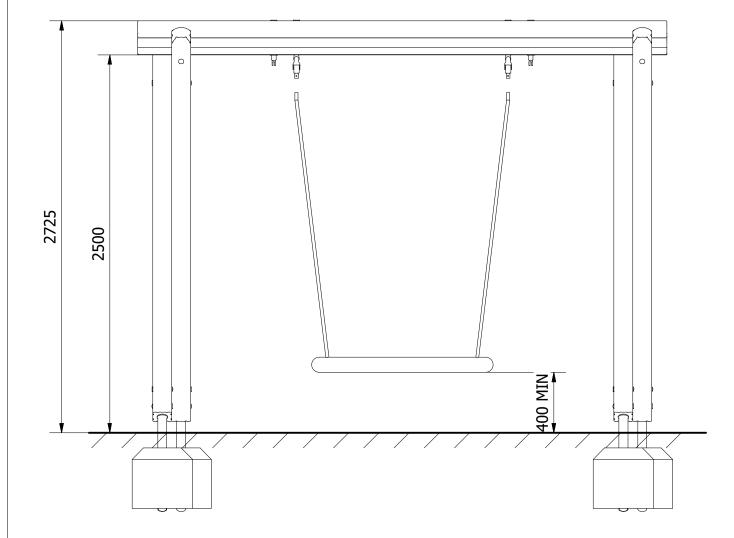
2. FINALLY, ENSURE UNIT IS LEVEL AND PLUMB, ALL FIXINGS HAVE BEEN TIGHTENED AND PROTECTIVE CAPS IN PLACE. ADD CONCRETE TO EACH FOUNDATION HOLE AND LEAVE FOR 48 HOURS
