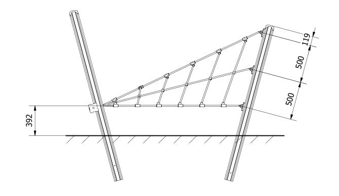
4. FINALLY, ENSURE ALL FIXINGS HAVE BEEN TIGHTENED AND PROTECTIVE CAPS IN PLACE, ADD CONCRETE TO EACH FOUNDATION HOLE AND LEAVE FOR 48 HOURS
