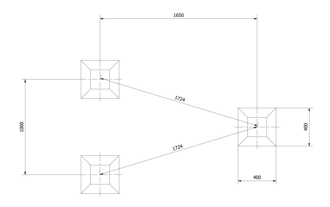
UNLESS OTHERWISE SPECIFIED: DIMENSIONS ARE IN MILLIMETERS TOLERANCES: LINEAR: ±2MM 1 DECIMAL PLACE: ±0.5MM ANGULAR: ±1°
