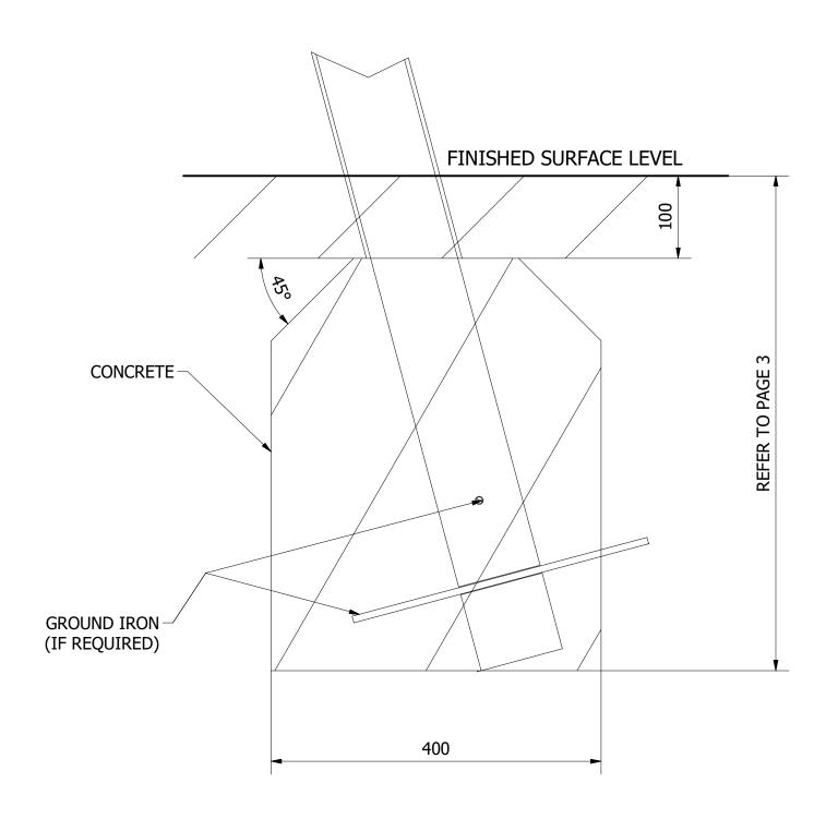
UNLESS OTHERWISE SPECIFIED: DIMENSIONS ARE IN MILLIMETERS THE INFORMATION CONTAINED IN THIS TOLERANCES: DRAWING IS THE SOLE PROPERTY OF FENLAND LEISURE PRODUCTS. ANY REPRODUCTION IN PART OR AS A WHOLE 1 DECIMAL PLACE: ±0.5MM WITHOUT THE WRITTEN PERMISSION ANGULAR: OF FENLAND LEISURE PRODUCTS IS PROHIBITED
