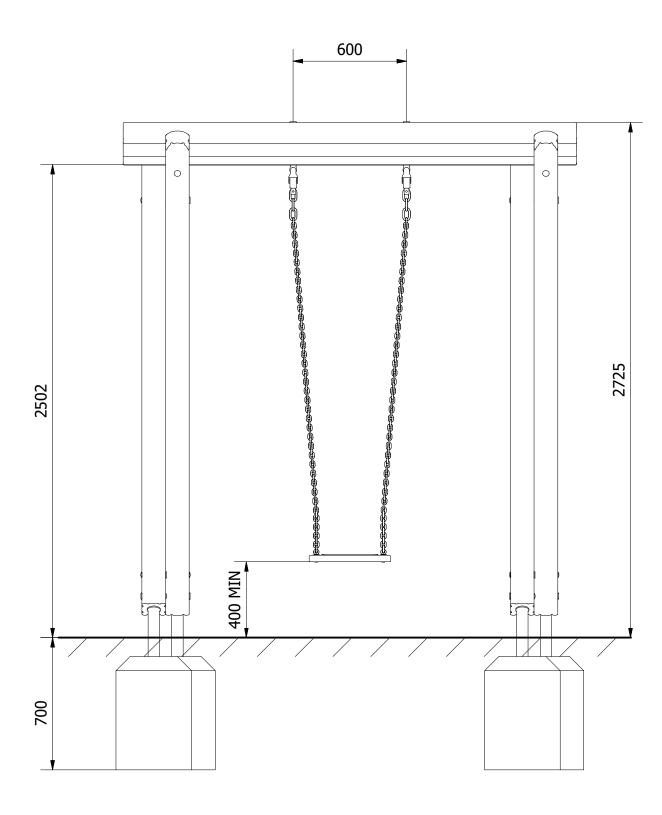
2. FINALLY, ENSURE UNIT IS LEVEL AND PLUMB, ALL FIXINGS HAVE BEEN TIGHTENED AND PROTECTIVE CAPS IN PLACE. ADD CONCRETE TO EACH FOUNDATION HOLE AND LEAVE FOR 48 HOURS
