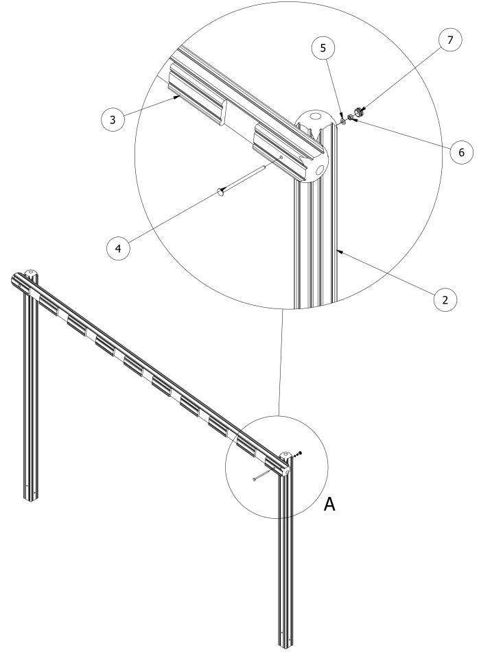
2. FINALLY, ENSURE THE UNIT IS LEVEL & PLUMB, ALL FIXINGS HAVE BEEN TIGHTENED AND PROTECTIVE CAPS IN PLACE. ADD CONCRETE TO THE FOUNDATION HOLE AND LEAVE FOR 48 HOURS
