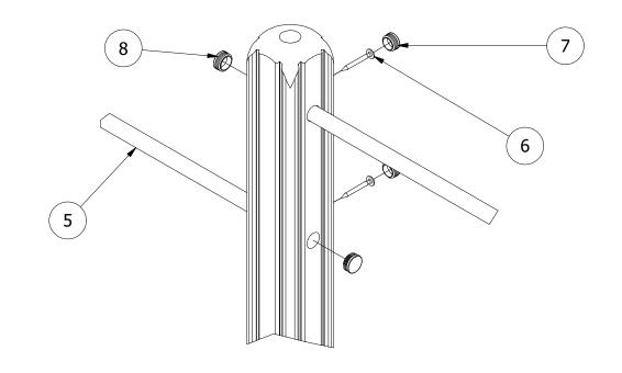
3. FINALLY, ENSURE ALL FIXINGS HAVE BEEN TIGHTENED AND PROTECTIVE CAPS IN PLACE. ADD CONCRETE TO EACH FOUNDATION HOLE AND LEAVE FOR 48 HOURS
