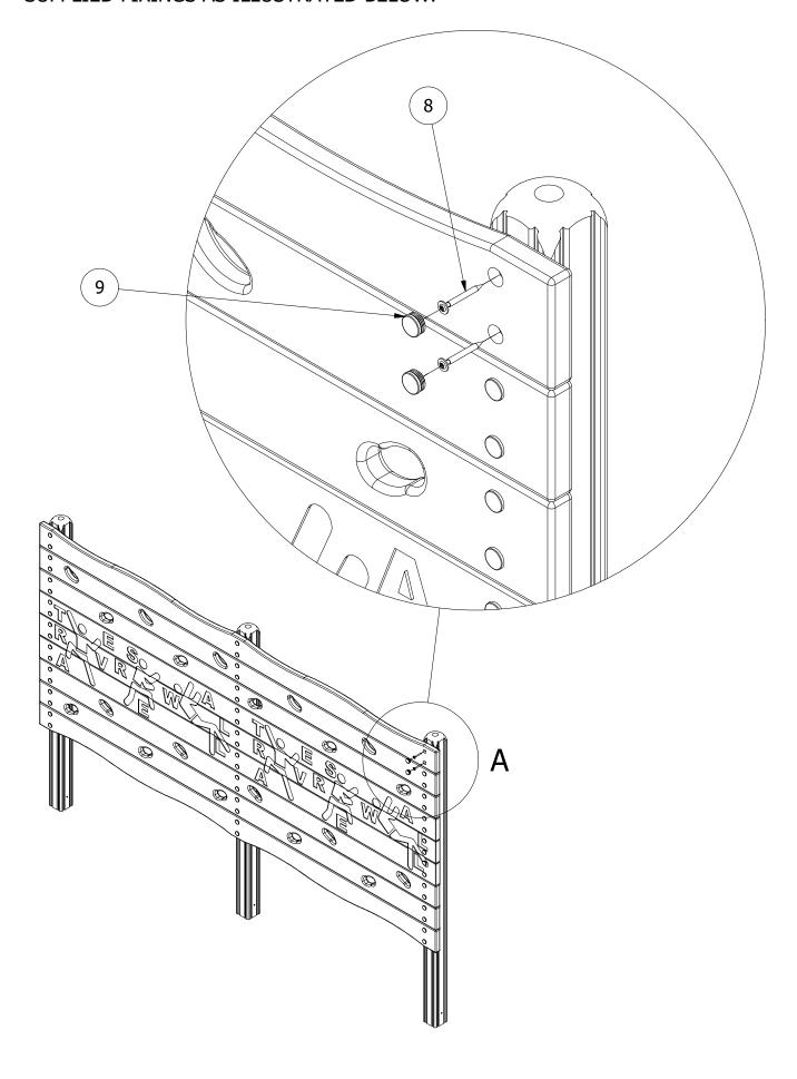
2. FINALLY, ENSURE UNIT IS LEVEL AND PLUMB, ALL FIXINGS HAVE BEEN TIGHTENED AND PROTECTIVE CAPS IN PLACE. ADD CONCRETE TO EACH FOUNDATION HOLE AND **LEAVE FOR 48 HOURS**
