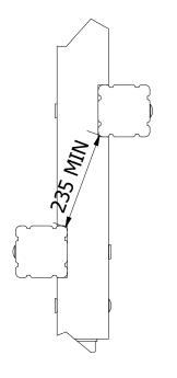
3. FINALLY, ENSURE THE UNIT IS LEVEL & PLUMB, ALL FIXINGS HAVE BEEN TIGHTENED AND PROTECTIVE CAPS IN PLACE. ADD CONCRETE TO THE REMAINING FOUNDATION HOLE AND LEAVE FOR 48 HOURS
