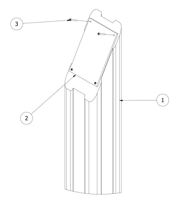
3. FINALLY, ENSURE ALL FIXINGS HAVE BEEN TIGHTENED AND PROTECTIVE CAPS IN PLACE. ADD CONCRETE TO EACH FOUNDATION HOLE AND LEAVE FOR 48 HOURS
