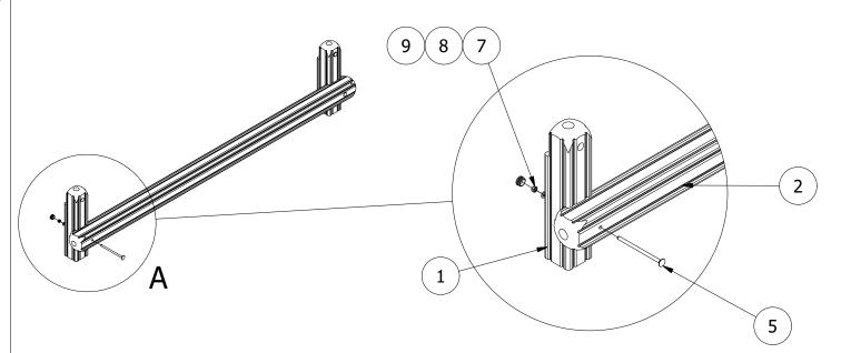
2. AS ILLUSTRATED BELOW, POSITION THE HORIZONTAL TIMBERS (ITEM 2), INTO THE CORRESPONDING REBATES IN THE UPRIGHT TIMBERS AND SECURE USING THE SUPPLIED THREADED BAR.
