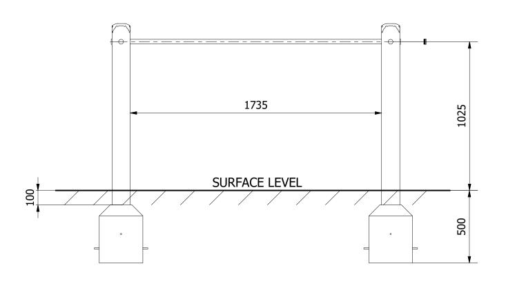
2. FINALLY, ENSURE UNIT IS LEVEL AND PLUMB, ALL FIXINGS HAVE BEEN TIGHTENED AND PROTECTIVE CAPS IN PLACE. ADD CONCRETE TO EACH FOUNDATION HOLE AND LEAVE FOR 48 HOURS
