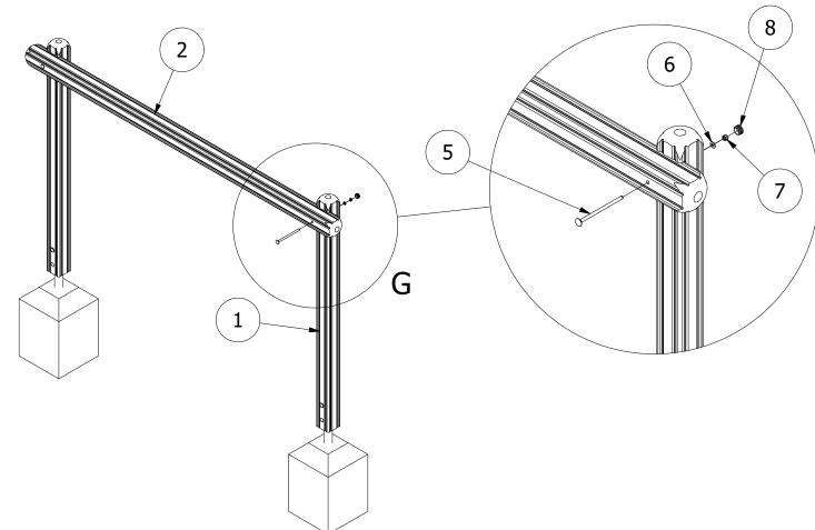
2. WITH THE TIMBERS CONNECTED AND BRACED, SECURE THE ROPE TO THE UPPER AND SIDE FRAME USING THE SUPPLIED FIXINGS AS ILLUSTRATED BELOW.
