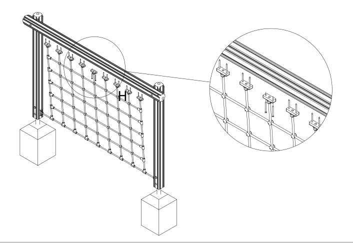
3. FINALLY, ENSURE ALL FIXINGS HAVE BEEN TIGHTENED AND PROTECTIVE CAPS IN PLACE. ADD CONCRETE TO EACH FOUNDATION HOLE AND LEAVE FOR 48 HOURS
