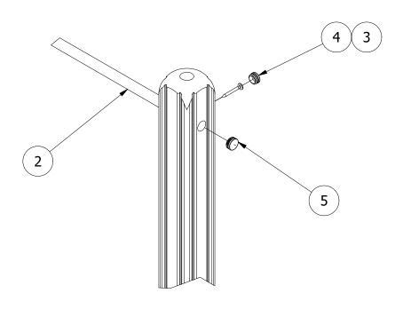
3. FINALLY, ENSURE ALL FIXINGS HAVE BEEN TIGHTENED AND PROTECTIVE CAPS IN PLACE. ADD CONCRETE TO EACH FOUNDATION HOLE AND LEAVE FOR 48 HOURS
