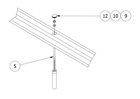
3. FINALLY, ENSURE THE UNIT IS LEVEL AND PLUMB, ALL FIXINGS HAVE BEEN TIGHTENED AND PROTECTIVE CAPS IN PLACE. ADD CONCRETE TO EACH FOUNDATION HOLE AND LEAVE FOR 48 HOURS
