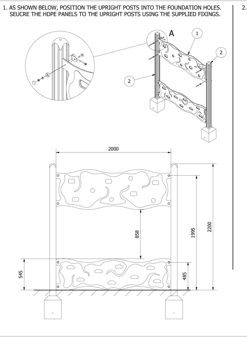
2. FINALLY, ENSURE THE UNIT IS LEVEL AND PLUMB. ALL FIXINGS HAVE BEEN TIGHTENED AND PROTECTIVE CAPS IN PLACE. ADD CONCRETE TO EACH FOUNDATION HOLE AND LEAVE FOR 48 HOURS.
