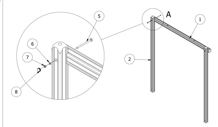
2. WITH THE MAIN FRAME IN PLACE, POSITION AND REMAINING POST INTO THE CENTRE OF THE UNIT. USE THE EYEBOLTS TO SECURE THE ROPE FROM THE TOP BAR, THEN ATTACH TO THE SIDE OF THE MAIN UPRIGHT, AND THE SIDE OF THE SMALLER STEPPING POST. **ENSURE ROPE IS TENSIONED**
