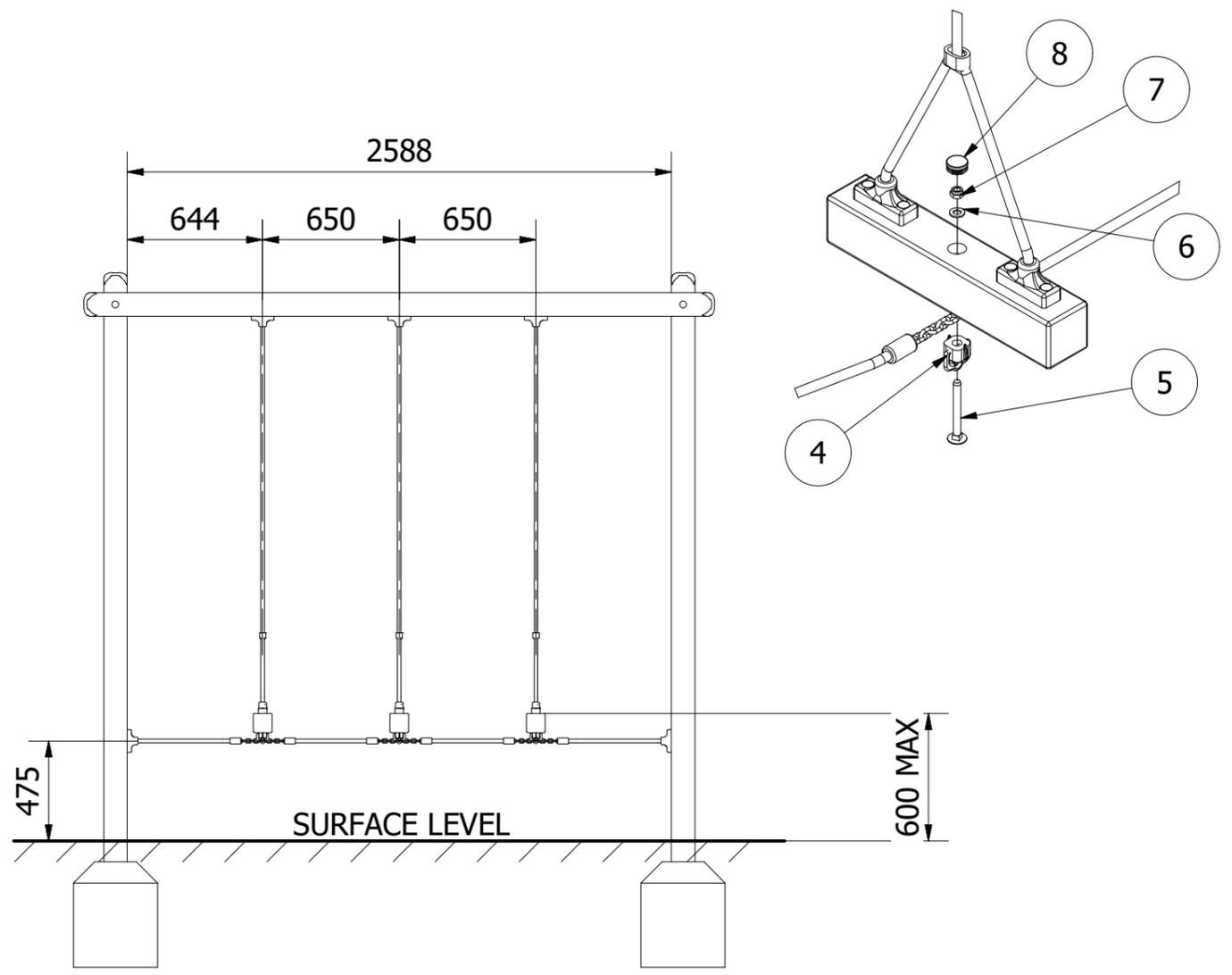
3. FINALLY, ENSURE UNIT IS LEVEL AND PLUMB, ALL FIXINGS HAVE BEEN TIGHTENED AND PROTECTIVE CAPS IN PLACE. ADD CONCRETE TO EACH FOUNDATION HOLE AND LEAVE FOR 48 HOURS
