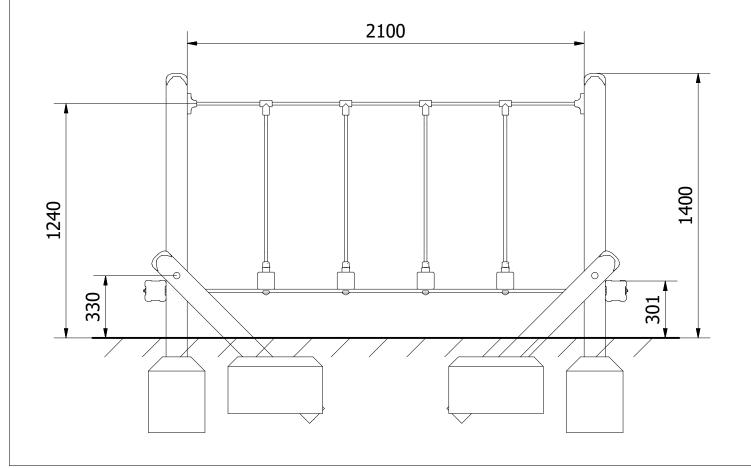
3. FINALLY, ENSURE UNIT IS LEVEL AND PLUMB, ALL FIXINGS HAVE BEEN TIGHTENED AND PROTECTIVE CAPS IN PLACE. ADD CONCRETE TO EACH FOUNDATION HOLE AND LEAVE FOR 48 HOURS
