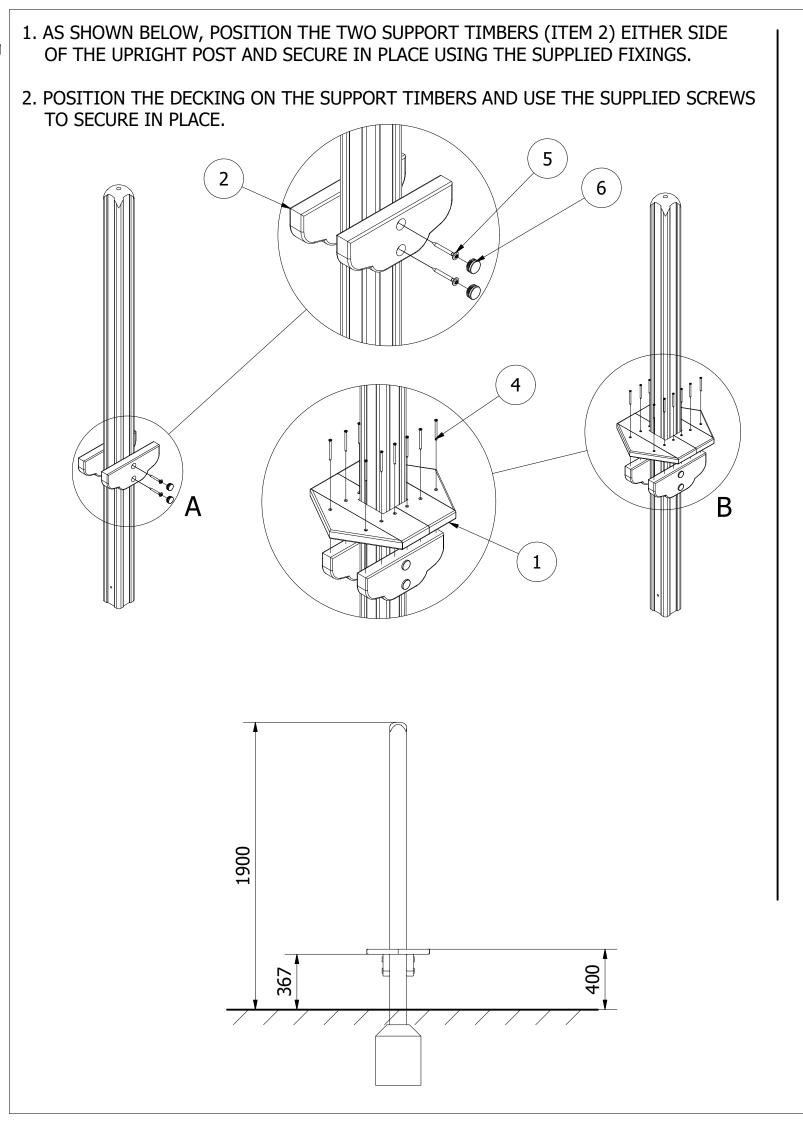
3. FINALLY, ENSURE THE UNIT IS LEVEL AND PLUMB. ALL FIXINGS HAVE BEEN TIGHTENED AND PROTECTIVE CAPS IN PLACE. ADD CONCRETE TO EACH FOUNDATION HOLE AND LEAVE FOR 48 HOURS.
