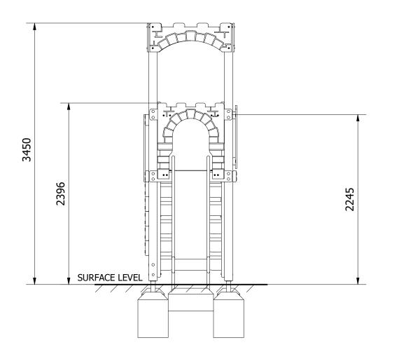
ENSURE UNIT IS LEVEL AND PLUMB, ALL FIXINGS HAVE BEEN TIGHTENED AND PROTECTIVE CAPS IN PLACE. ADD CONCRETE TO EACH FOUNDATION HOLE AND LEAVE FOR 48 HOURS.
