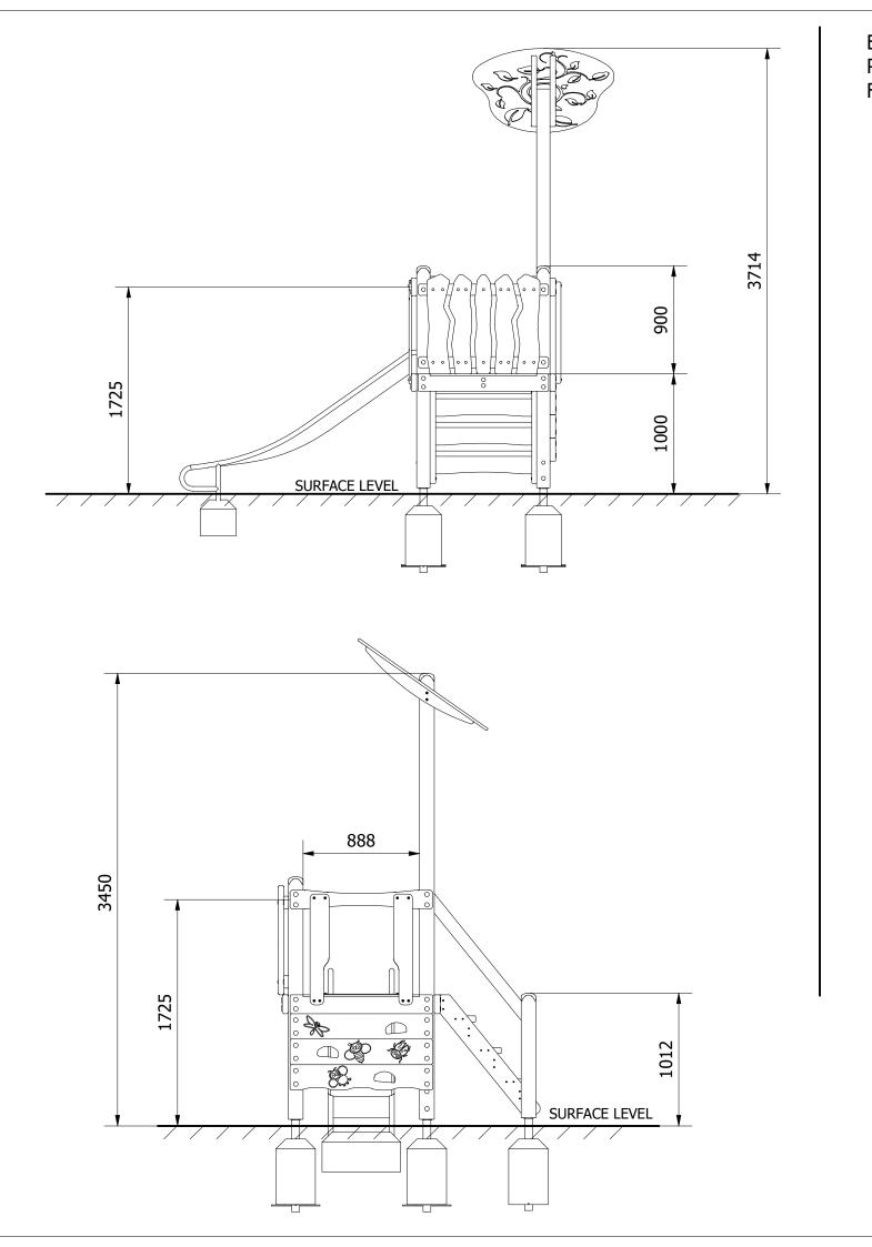
ENSURE UNIT IS LEVEL AND PLUMB, ALL FIXINGS HAVE BEEN TIGHTENED AND PROTECTIVE CAPS IN PLACE. ADD CONCRETE TO EACH FOUNDATION HOLE AND LEAVE FOR 48 HOURS.
