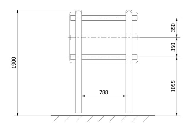
3. FINALLY, ENSURE ALL FIXINGS HAVE BEEN TIGHTENED AND PROTECTIVE CAPS IN PLACE. ADD CONCRETE TO EACH FOUNDATION HOLE AND LEAVE FOR 48 HOURS
