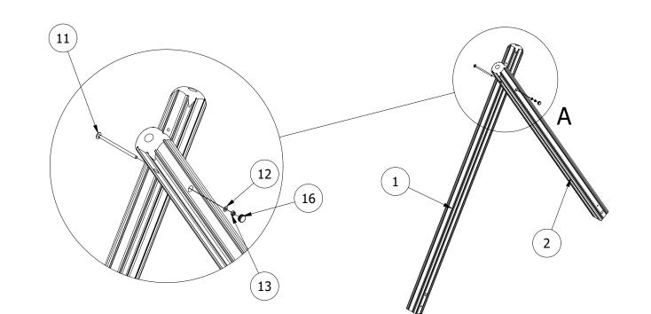
2. POSITION THE A-FRAMES INTO THE FOUNDATION HOLES AND BRACE. (TAKE NOTE OF THE POSITION OF THE POSTS AS SHOWN IN FIG 1) POSITION THE TOP BAR ONTO THE A-FRAMES AND SECURE IN PLACE.
