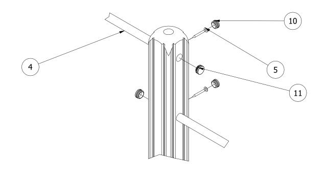
3. FINALLY, ENSURE ALL FIXINGS HAVE BEEN TIGHTENED AND PROTECTIVE CAPS IN PLACE. ADD CONCRETE TO EACH FOUNDATION HOLE AND LEAVE FOR 48 HOURS
