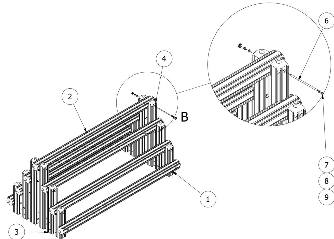
3. FINALLY, ENSURE UNIT IS LEVEL AND PLUMB, ALL FIXINGS HAVE BEEN TIGHTENED AND PROTECTIVE CAPS IN PLACE. ADD CONCRETE TO EACH FOUNDATION HOLE AND LEAVE FOR 48 HOURS
