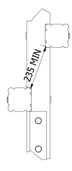
3. FINALLY, ENSURE THE UNIT IS LEVEL & PLUMB, ALL FIXINGS HAVE BEEN TIGHTENED AND PROTECTIVE CAPS IN PLACE. ADD CONCRETE TO THE REMAINING FOUNDATION HOLE AND LEAVE FOR 48 HOURS
