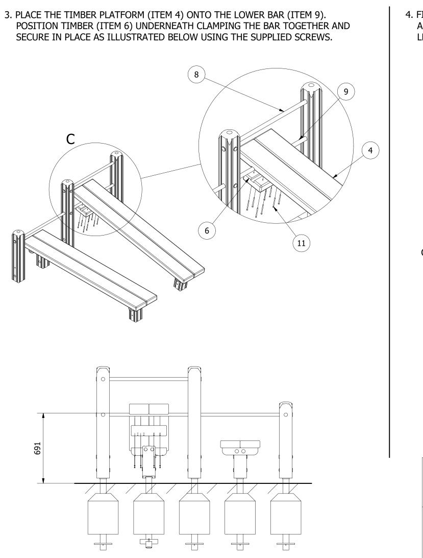
4. FINALLY, ENSURE UNIT IS LEVEL AND PLUMB, ALL FIXINGS HAVE BEEN TIGHTENED AND PROTECTIVE CAPS IN PLACE. ADD CONCRETE TO EACH FOUNDATION HOLE AND LEAVE FOR 48 HOURS
