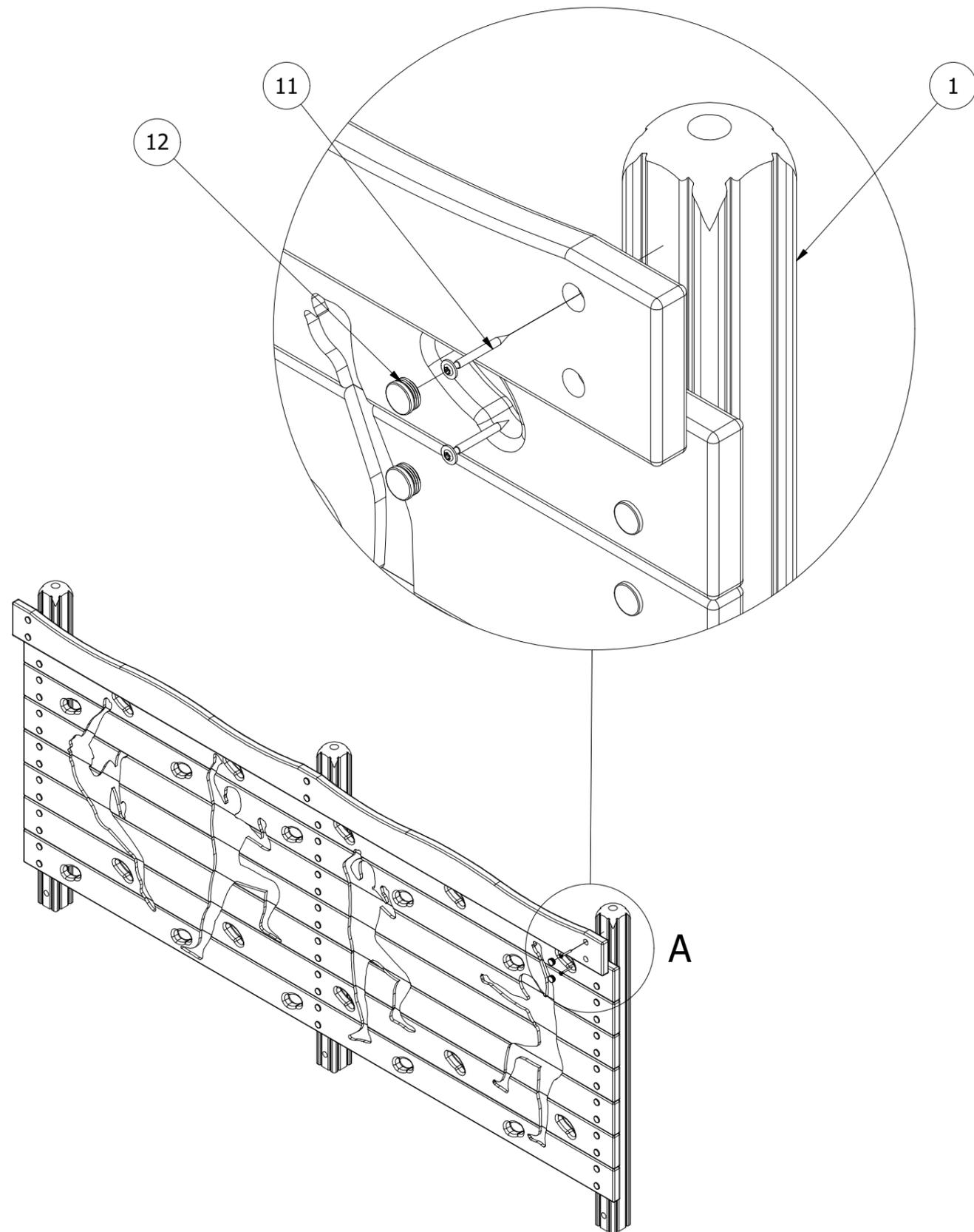
2. FINALLY, ENSURE UNIT IS LEVEL AND PLUMB, ALL FIXINGS HAVE BEEN TIGHTENED AND PROTECTIVE CAPS IN PLACE. ADD CONCRETE TO EACH FOUNDATION HOLE AND LEAVE FOR 48 HOURS
