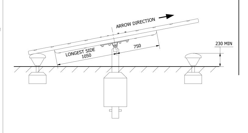
3. FINALLY, ENSURE UNIT IS LEVEL AND PLUMB, ALL FIXINGS HAVE BEEN TIGHTENED AND PROTECTIVE CAPS IN PLACE. ADD CONCRETE TO EACH FOUNDATION HOLE AND LEAVE FOR 48 HOURS
