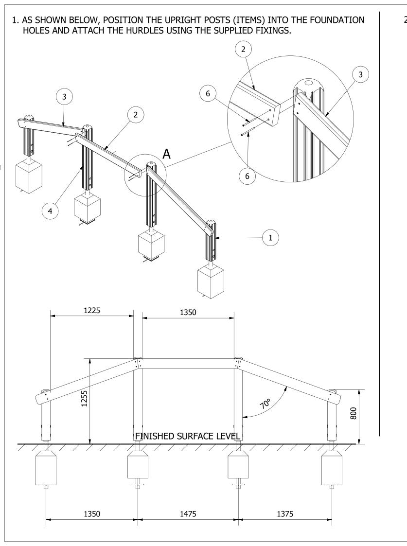
2. FINALLY, ENSURE THE UNIT IS LEVEL AND PLUMB. ALL FIXINGS HAVE BEEN TIGHTENED AND PROTECTIVE CAPS IN PLACE. BRACE & ADD CONCRETE TO EACH FOUNDATION HOLE AND LEAVE FOR 48 HOURS
