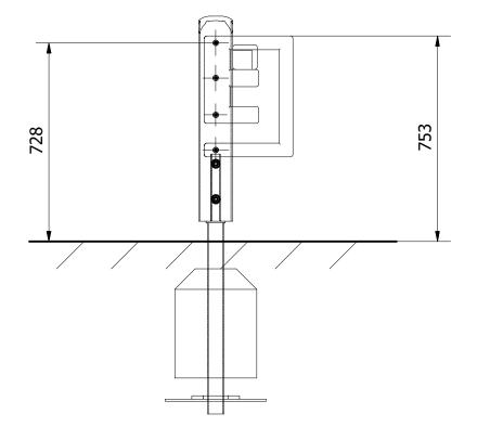
3. FINALLY, ENSURE THE UNIT IS LEVEL AND PLUMB. ALL FIXINGS HAVE BEEN TIGHTENED AND PROTECTIVE CAPS IN PLACE. ADD CONCRETE TO EACH FOUNDATION HOLE AND LEAVE FOR 48 HOURS
