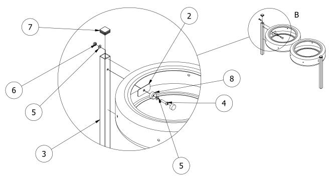
4. FINALLY, ENSURE THE UNIT IS LEVEL AND PLUMB. ALL FIXINGS HAVE BEEN TIGHTENED AND PROTECTIVE CAPS IN PLACE. ADD CONCRETE TO EACH FOUNDATION HOLE AND LEAVE FOR 48 HOURS.
