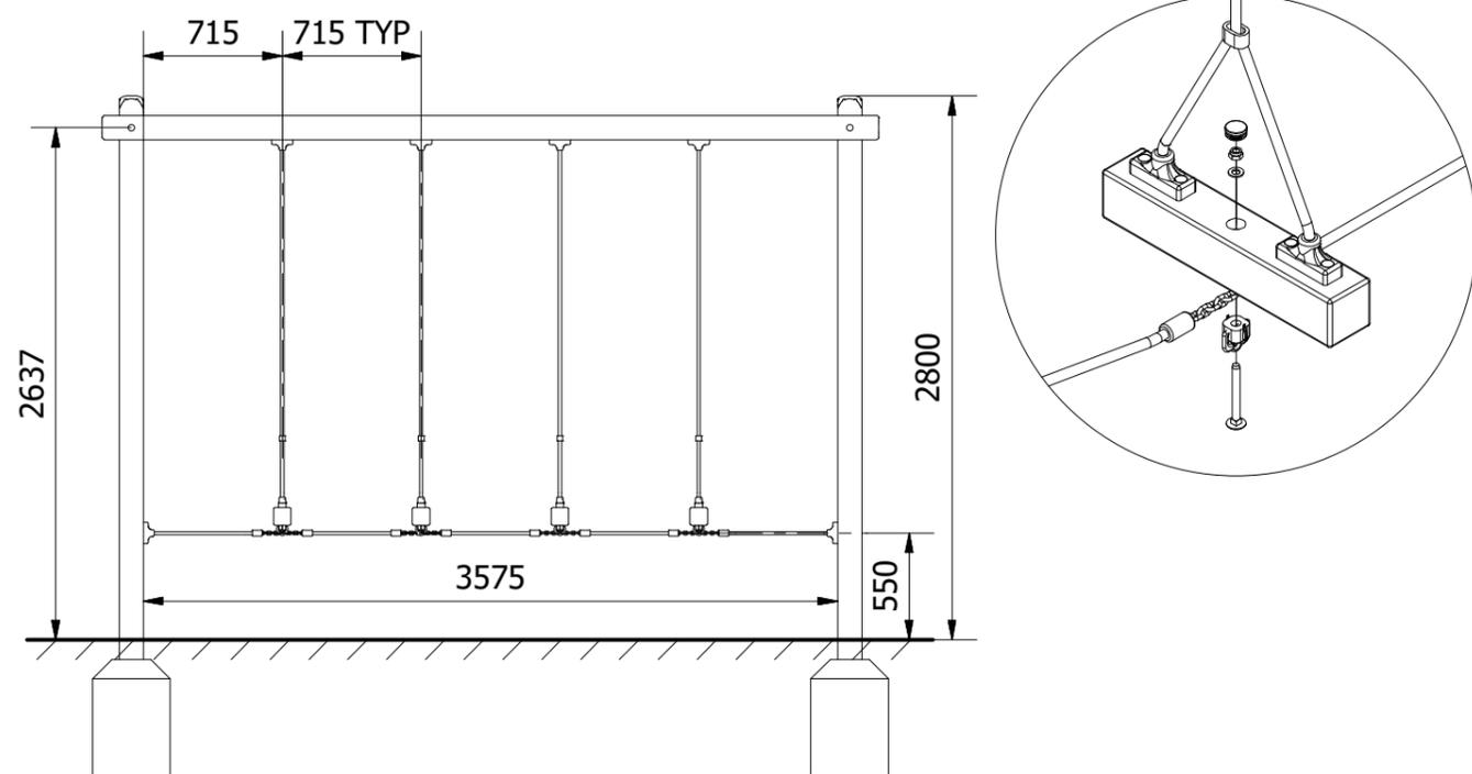
3. FINALLY, ENSURE ALL FIXINGS HAVE BEEN TIGHTENED AND PROTECTIVE CAPS IN PLACE.
