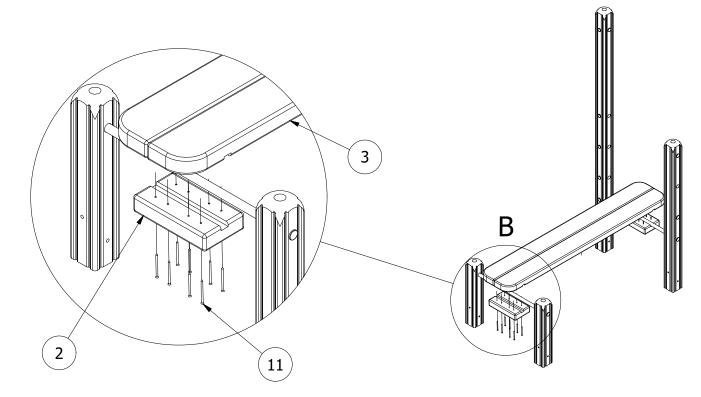
3. FINALLY, ENSURE THE UNIT IS LEVEL & PLUMB. ALL FIXINGS HAVE BEEN TIGHTENED AND PROTECTIVE CAPS IN PLACE. ADD CONCRETE TO EACH FOUNDATION HOLE AND LEAVE FOR 48 HOURS
