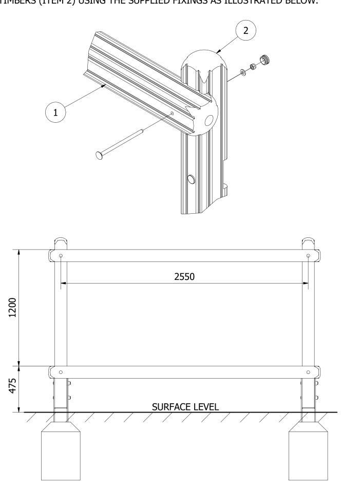
3. FINALLY, ENSURE THE UNIT IS LEVEL & PLUMB, ALL FIXINGS HAVE BEEN TIGHTENED AND PROTECTIVE CAPS IN PLACE. ADD CONCRETE TO THE REMAINING FOUNDATION HOLE AND LEAVE FOR 48 HOURS
