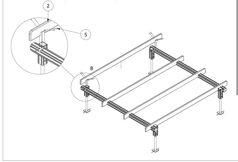
3. FINALLY, ENSURE ALL FIXINGS HAVE BEEN TIGHTENED AND PROTECTIVE CAPS IN PLACE.
