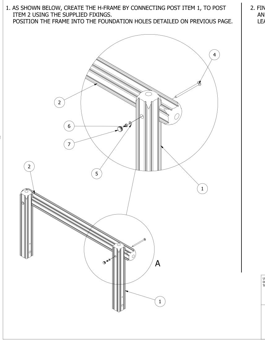
2. FINALLY, ENSURE THE UNIT IS LEVEL & PLUMB, ALL FIXINGS HAVE BEEN TIGHTENED AND PROTECTIVE CAPS IN PLACE. ADD CONCRETE TO THE FOUNDATION HOLE AND **LEAVE FOR 48 HOURS**
