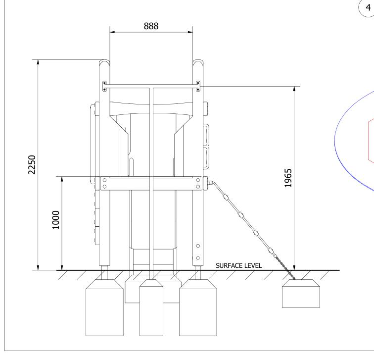
Title: UNLESS OTHERWISE SPECIFIED: DIMENSIONS ARE IN MILLIMETERS TOLERANCES: PROPRIETARY AND CONFIDENTIAL THE INFORMATION CONTAINED IN THIS DRAWING IS THE SOLE PROPERTY OF FENLAND LEISURE PRODUCTS. ANY REPRODUCTION IN PART OR AS A WHOLE WITHOUT THE WRITTEN PERMISSION OF FENLAND LEISURE PRODUCTS IS PROHIBITED. LINEAR: ±2MM 1 DECIMAL PLACE: ±0.5MM ANGULAR: ±1° Produc online playgrounds
