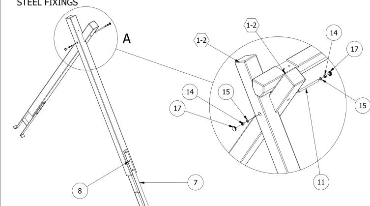
2. POSITION THE A-FRAMES INTO THE FOUNDATION HOLES AND BRACE. (TAKE NOTE OF THE POSITION OF THE POSTS AS SHOWN IN FIG 1) POSITION THE TOP BAR ONTO THE A-FRAMES AND SECURE IN PLACE.
