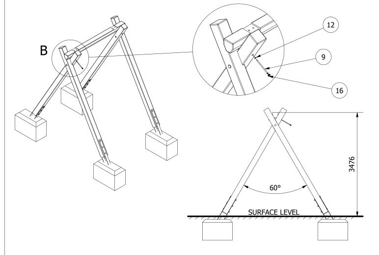
3. WITH BOTH FRAMES POSITIONED AND PROPPED IN THE FOUNDATION HOLES, POSITION THE MAIN SWING BEAM ONTO THE TOP A-FRAME BAR. USE THE SUPPLIED BOLTS TO SECURE.
