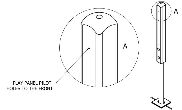
2. POSITION THE SECOND POST INTO THE FOUNDATION HOLE AS ILLUSTRATED BELOW.
